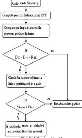
Fig1.Path Tracing Algorithm.
