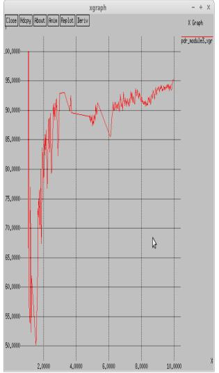
Fig5.Graph depicting Packet delivery Ratio where x-axis denotes normal time in ms and y-axis denotes delivery ratio.
