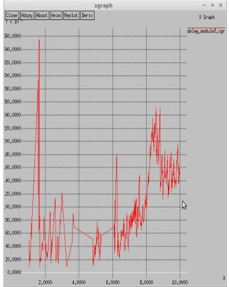
Fig6. Depicting the delay with x-axis denotes normal time and y-axis denotes delay in millisecs.
